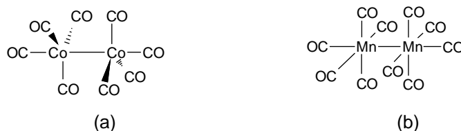
Figure 13.4 The metal–metal bonds of (a) \text{Co}_2(\text{CO})_8 and (b) \text{Mn}_2(\text{CO})_{10} give the metal atoms stable electronic configurations with 18 electrons in the outer shell
